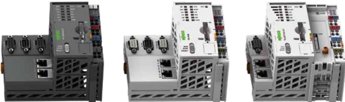
The impressive PFC200 Controller features high processing speed and a large selection of interfaces. The CANopen, PROFIBUS DP and Modbus TCP/UDP/RTU protocols provide flexible connection to fieldbus systems and external input/output devices. And multiple variants – one with an integrated wireless modem and the robust, expanded temperature range (XTR Series) – provide these features for virtually any application.
